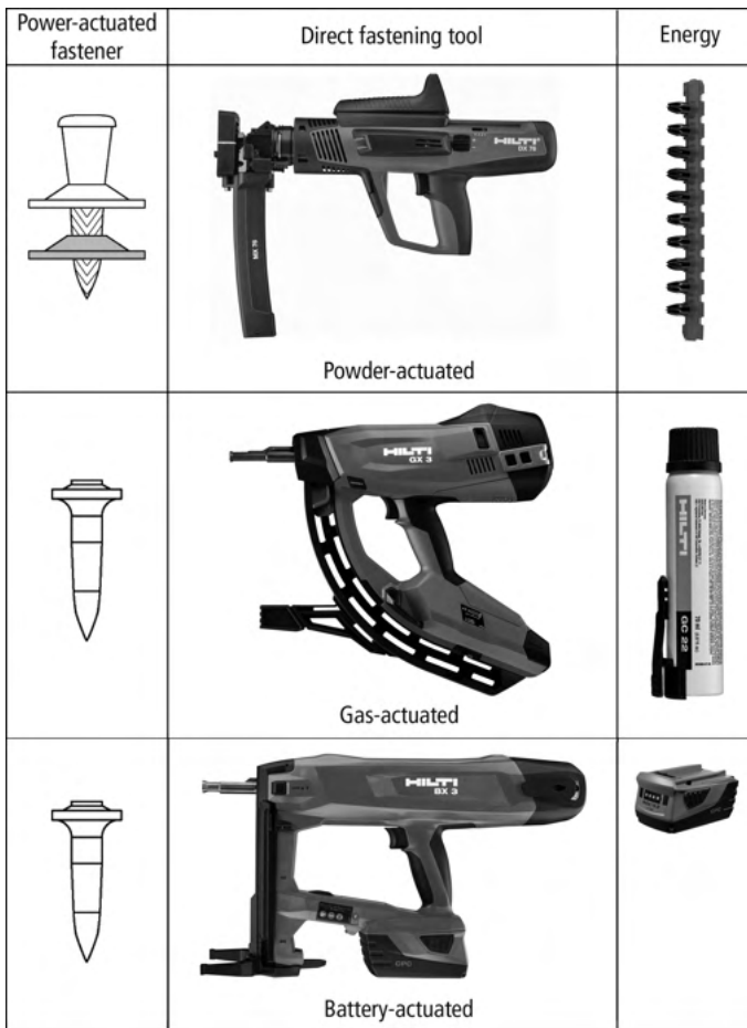
Figure 3. Components of direct fastening systems
