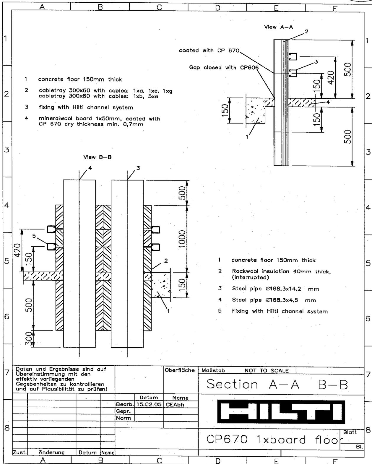
Figure 3 Diagram showing details of penetrating services passing through seal A.
