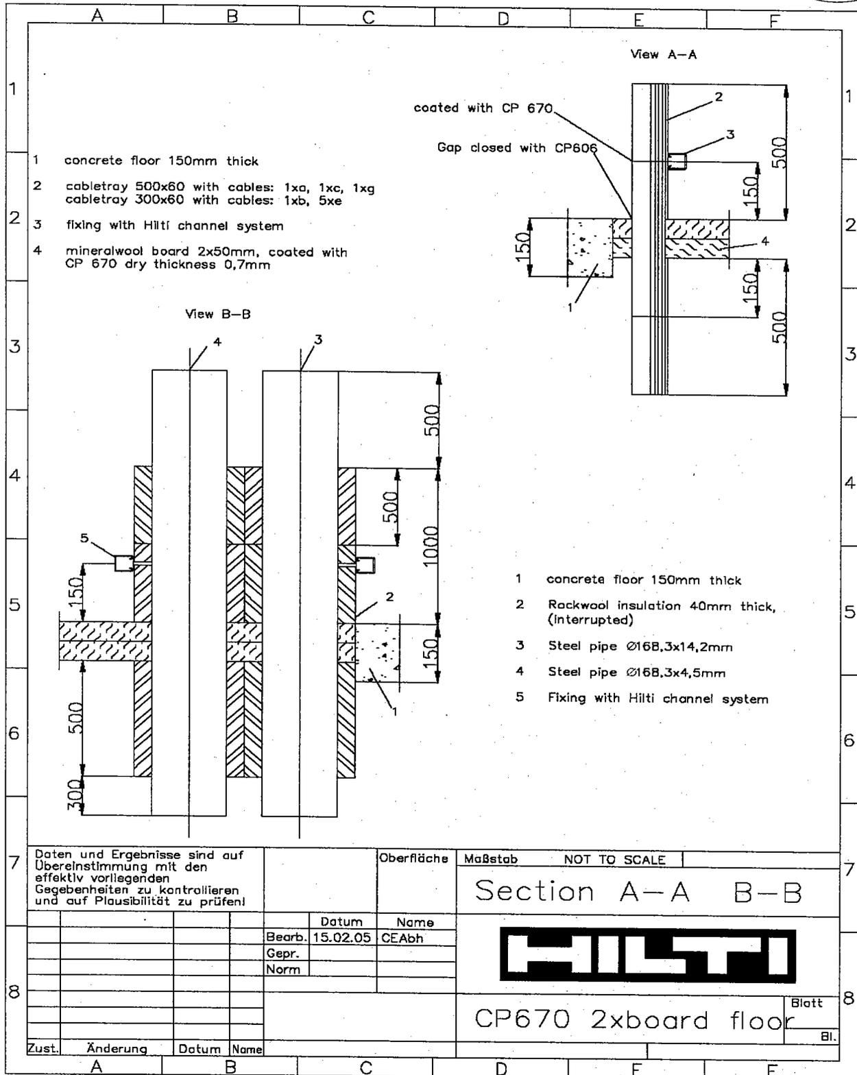
Figure 6 Diagram showing details of penetrating services passing through seal B
