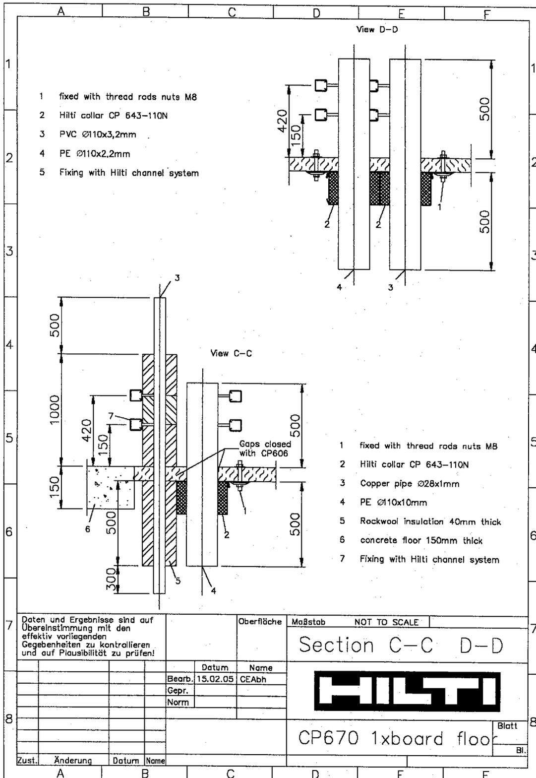
Figure 4 Diagram showing detail of penetrating services passing through seal A.
