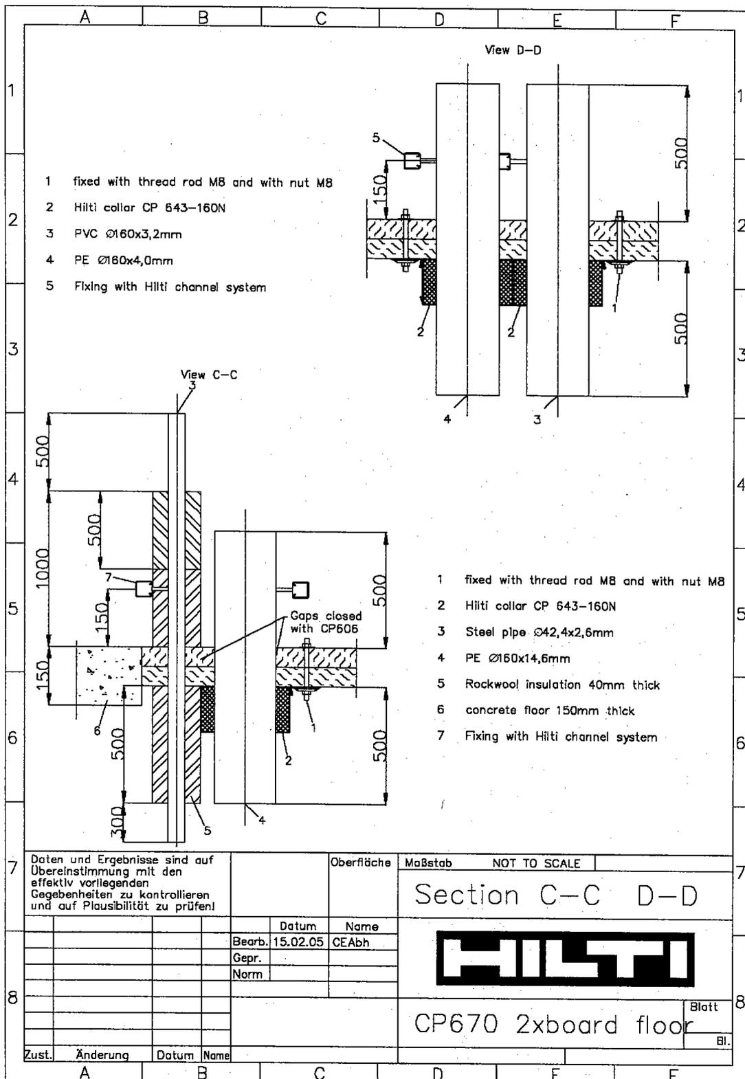
Figure 7 Diagram showing details of penetrating services passing through seal B
