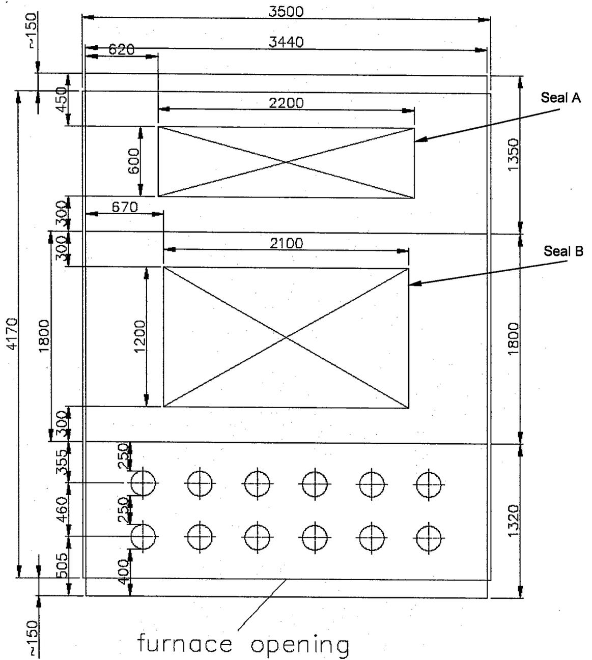
Figure 1 Diagram showing the position of the floor slabs as installed within the test frame.
