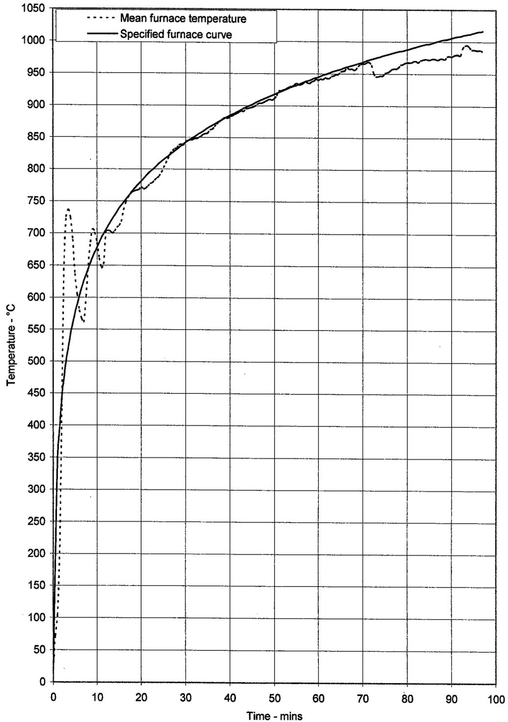
**Graph 1** Mean furnace temperature with the specified furnace curve for comparison.
