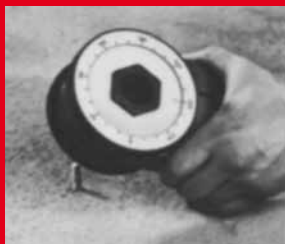
The gauge can be connected straight to the HSA (HKB), HVA (adhesive) and HSLG heavy-duty stud anchor. The central bore is placed over the protruding threaded section of the anchor.
